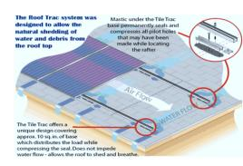
Roof Top Flush Mounting System
